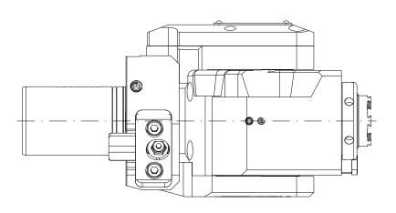
n1(max) = 6500 U/min n2(max) = 6500 U/min M (max) = 24 Nm
